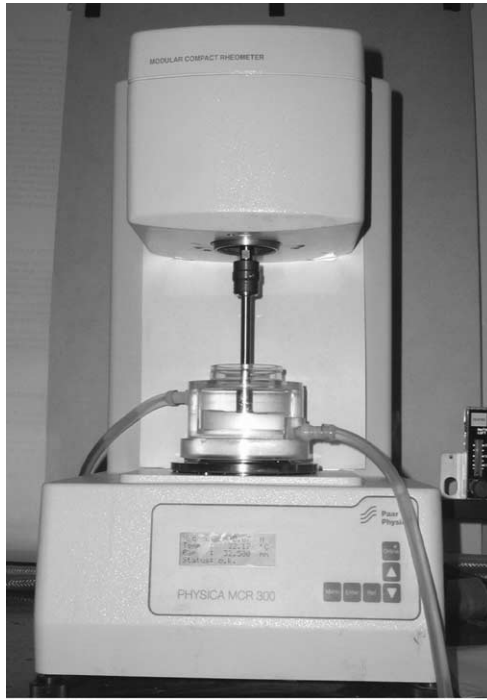
Fig. 1. Photograph showing the adaptations made to the conventional rheometer and schematic diagram showing the physical dimensions of the measuring system (biconical disk and containing vessel). R_b : radius of biconical disk, R_c : radius of vessel, \alpha : half angle of biconical disk, H_1 : depth of fluid 1, H_2 : depth of fluid 2.
